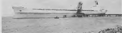
The 88,000 dwt. tanker "Jacob Maersk" is the largest tanker to dock at Lago's new Sea Berth. Arriving May 16, she loaded 570,000 barrels of fuel oil, and sailed the next day for Melford Haven, England.
